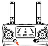
**METHOD 2:** The Drone will automatically lock if there is no operation detected for **15 seconds** after unlocking or landing.
